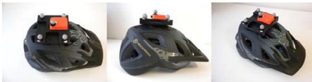
Fig. 3 Bike helmet with MTx unit and some VICON markers
